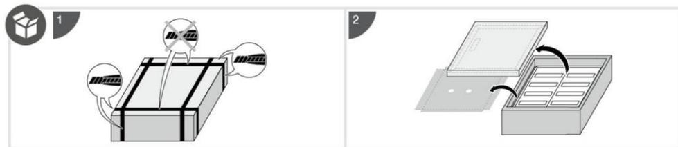
Well-thought-out packaging for the FWU field distributor: full plaster guard, separate packaging of frame and door for secure intermediate storage
