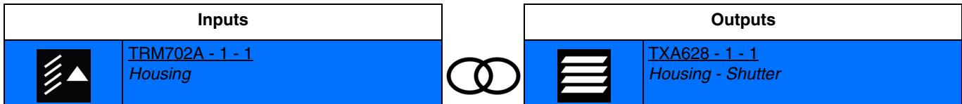
Activating the input by a short press briefly closes the Up output contact (function direction of a blind's slats).
