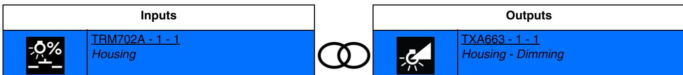
Activating the input switches the light on to the brightness value defined.
