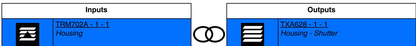
Activating the input closes the Up output contact for a length of time (function raising a rolling shutter or a blind).
