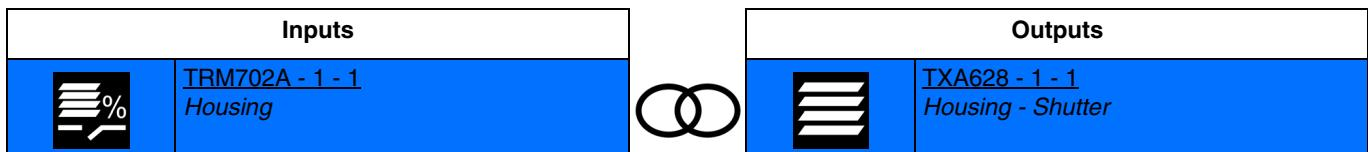
Closing input contact: delayed closing of output contacts for position 1 of the shutter or blind.
