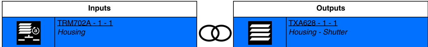
Activating the input closes the output contacts for positioning the shutter or blind for a length of time.
