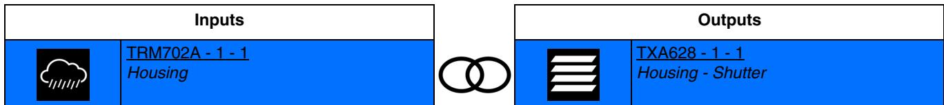
Closing input contact: rain alarm activation.
