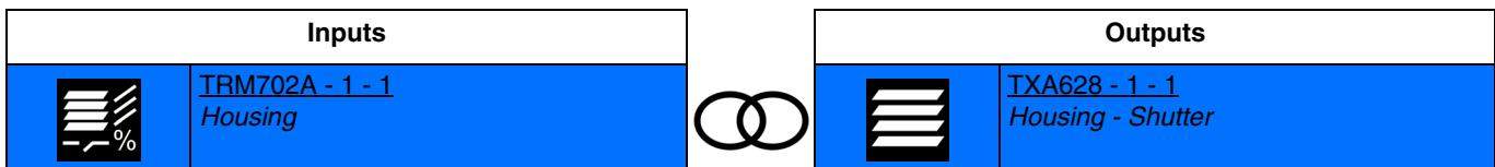
Closing input contact: delayed closing of output contacts for position 1 of the shutter or blind and for position 1 for blind slats.
