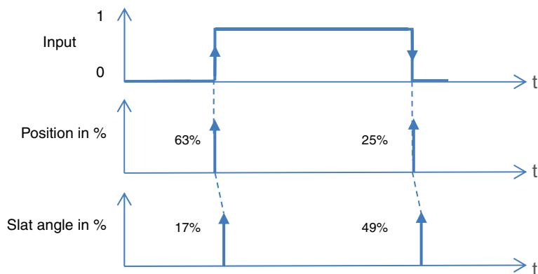
Note: The value of the object **Position in %** is issued before the object value **Slat angle in %** so that the output module can position the blind before tilting it.
