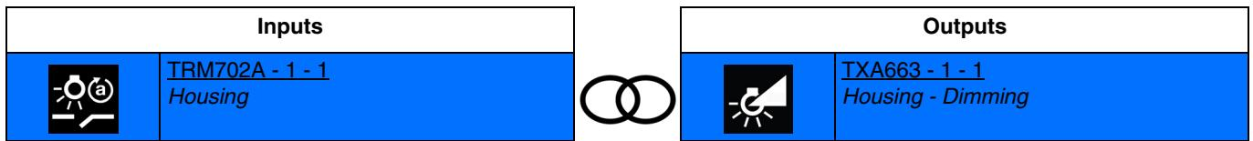
Closing input contact: turns on the light at the 1 brightness value.
