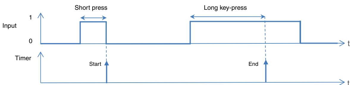
The Timer function is used to switch on a lighting circuit for a programmable period.
