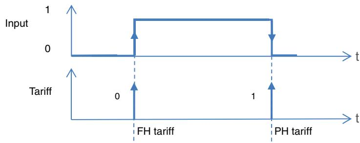
*Note: By default, the input operates like an NO contact (Normally open). If the parameter **Inverted** is validated, the input operates like an NC contact (Normally closed).*
