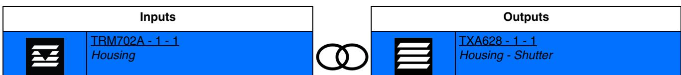
Activating the input closes the Down output contact for a length of time (Function Lowering a rolling shutter or a blind).
