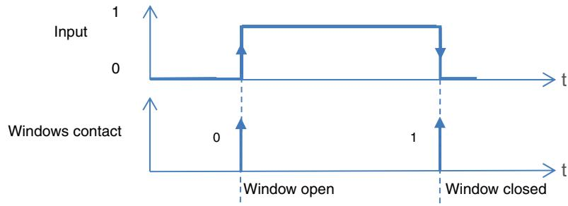
*Note: By default, the input operates like an NO contact (Normally open). If the parameter **Inverted** is validated, the input operates like an NC contact (Normally closed).*
