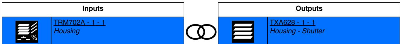
Activating the input closes the output contacts for positioning the shutter or blind and for tilting the blind slats for a length of time.
