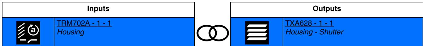
Closing input contact: delayed closing of output contacts for position 1 of the blind slats.
