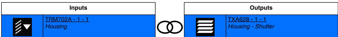
Activating the input by a short press briefly closes the Down output contact (function direction of a blind's slats).
