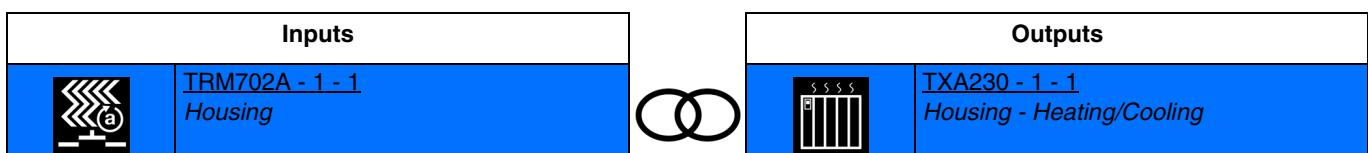
Closing the input contact activates heating mode 1.
