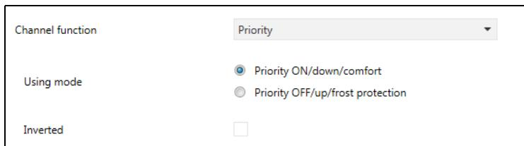
The Priority function is used to force the output into a defined state.
