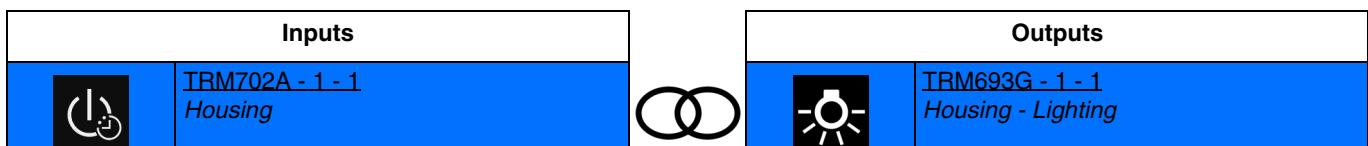
Activating the input by a short press <1 s switches on the light for a length of time.
