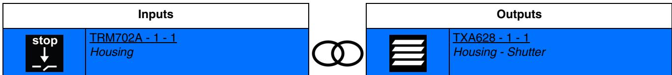
Closing input contact: delayed closing of the lowering output contact.
