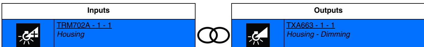
Activating the input by short presses switches on the light to the last level memorised.
