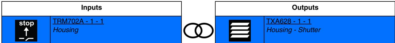
Closing input contact: delayed closing of the raise output contact.
