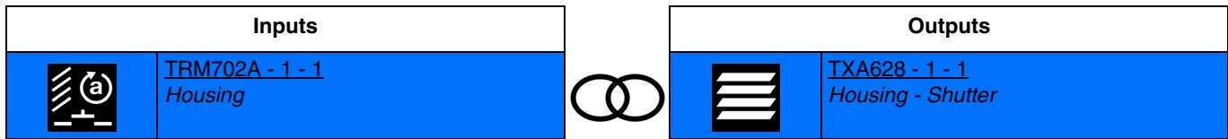
Activating the input closes the output contacts for tilting the blind slats for a length of time.
