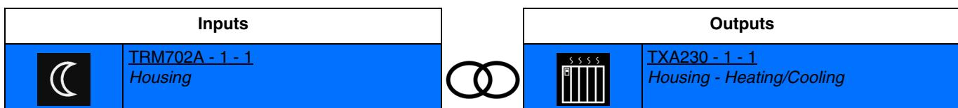
Closing the input contact activates Eco mode.
