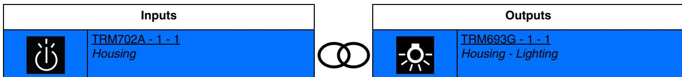
Activation of the input by short presses switches on the light.
