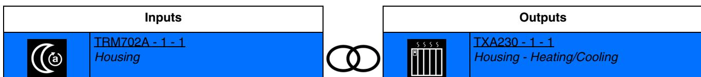
Closing the input contact activates Eco mode.
