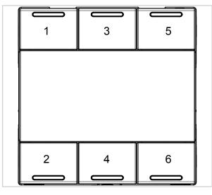
Figure 2: Button/input assignment – numbering in configuration tool
