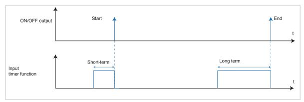
Figure 21: Signal-time diagram for timer
