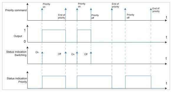
Figure 24: Signal-time diagram for Priority
