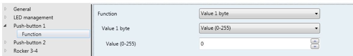
Figure 26: Function of the "Value 1 byte" independent push-button
