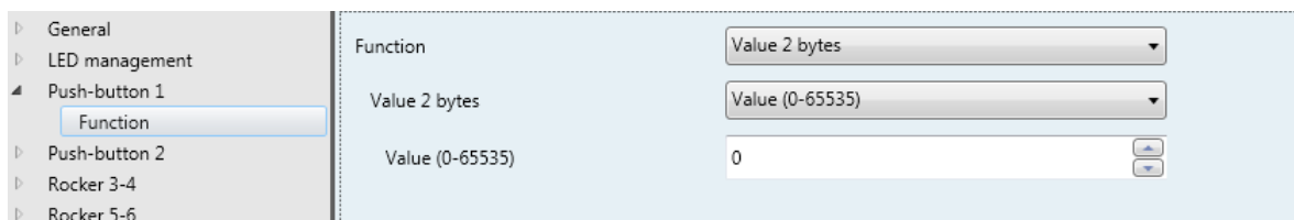
Figure 27: Function of the "Value 2 bytes" independent push-button
